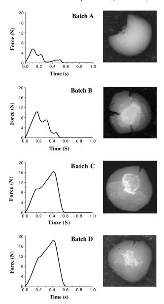
Fig. 2. Examples of crushing strength plots and the corresponding images of the crushed pellets for the four batches of pellets. Images were taken after the first peak or notch.
