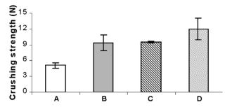
Fig. 3. Crushing strength of the four batches of pellets.
